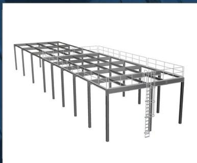
*Machine platform with railing and ladder. The support posts are only placed on the exterior edges of the footprint, so that the space under the platform can be used without interference.*
