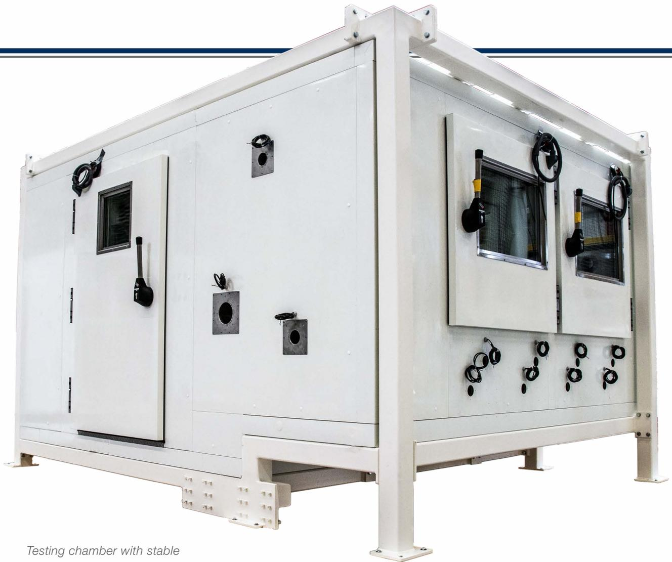
*Testing chamber with stable exterior construction made of steel profiles*
