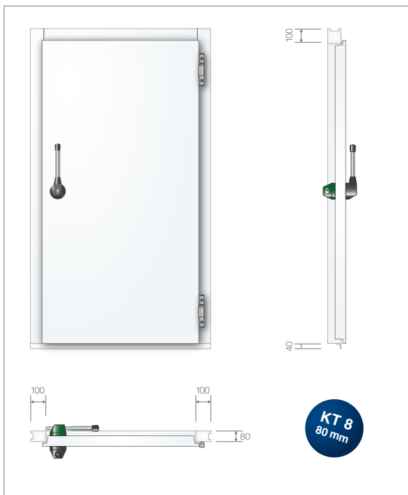
Chiller chamber door KT 8 80 mm insulation thickness, +25°C to 0°C Standard block frame for installation in masonry
